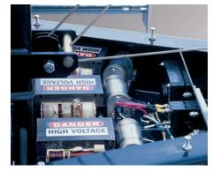
Each floodlight requires a ballast for starting. They are built into the tongue of the trailer in an easy to service weather resistant compartment. An internal fan ensures proper cooling. The light control panel is positioned outside the compartment and contains (2) single-pole 20A ON/OFF circuit breakers.
