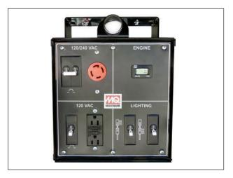
The LT6K offers a versatile control box that features: an Hour Meter, (1) NEMA L14-30R twist lock 120/240VAC 30A receptacle, (1) duplex GFCI 120VAC 15A receptacle, support circuit breakers, and panel light.
