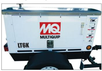
Ease of control panel operations, scheduled maintenance, and serviceability is supported by oversized (20"x41") access doors with lockable door handle and hood locking latches.
